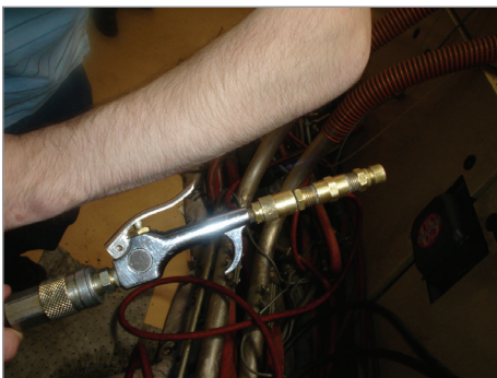
Venturi nozzles on blow guns can reduce compressed air consumption by 50-75%.
